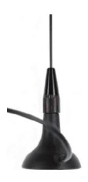
The mobile antenna is designed for installation on a vehicle or on a metal surface. The magnetic attachment system is easy to remove. It does not require drilling, the cable being positioned on the side. It comes with its mounting system and with its 3m cable with SMA male connector.
