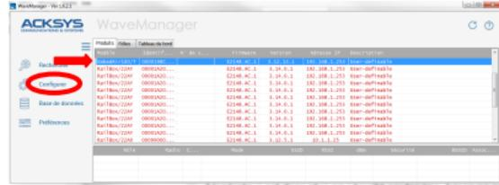
Else, select the device and click on « **Configure** » button. You can configure the IP address to make it accessible in your network or activate the DHCP client.
