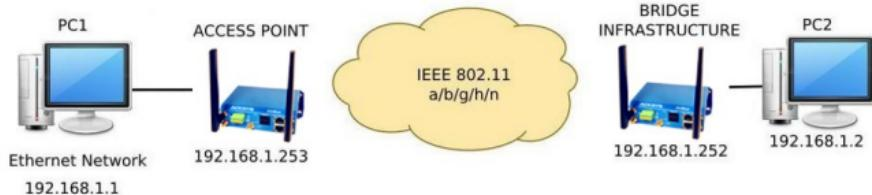
Set up the IP addresses according to the picture above and set the device connected to PC2 to Client (infrastructure) role.
