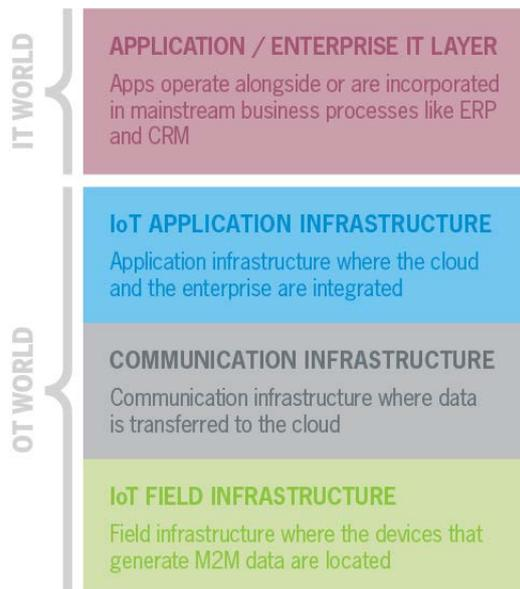
If we now focus on the communication infrastructure, then it is clear that south-facing protocols and interfaces are needed to communicate with the field infrastructure, as well as north-facing Internet connectivity technologies that communicate with the cloud.
