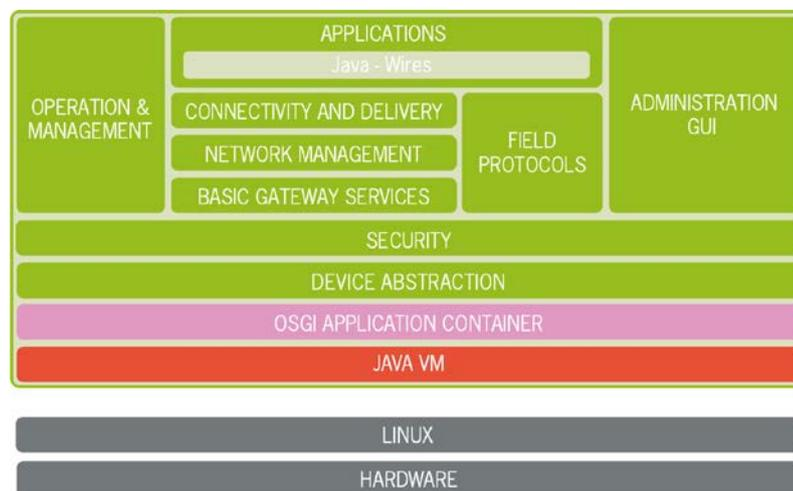
Figure 8. ESF enables wide, deep, seamless integration of applications with the operating system (Linux) and the hardware (devices), while providing full flexibility in terms of programming.
