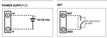
(\*) Note: for UL installation the device must be powered using a power supply unit classified NEC class 2 or SELV
