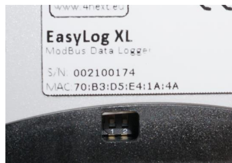
Fig. 6 Example DIP-SWITCH OFF position
