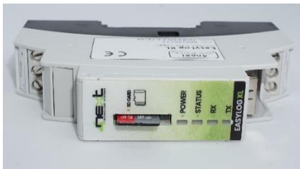
Fig.1 SD Card insert
