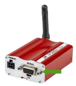
The RB900-Pro terminal is equipped with a D-Sub DE15F 15-pin connector to control the RS232 interface, RS232 AUX/Debug/MCU/Modem (option) or RS485 Modem/MCU (option).
