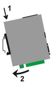
Removing the unit from the DIN rail
