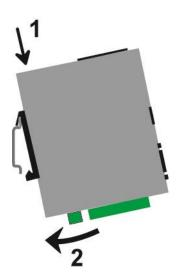
Removing the unit from the DIN rail
